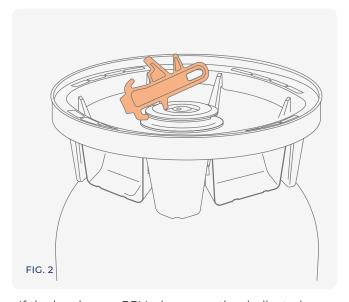
If the keg has no PRV, please use the dedicated depressurization key. It is suitable for all types of PolyKeg@ valves: A, D, G, K, M, S.
