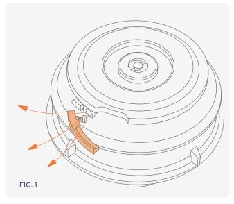
Once tapped, the empty keg must be depressurized immediately by breaking of the red PRV — pressure relief valve - lever.
